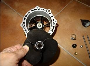
Security insert have function to prevent unscrewing of the impeller. Note alignment.
