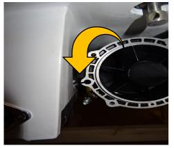
Remove jet pump stator – just wiggle and pull. Now stator is free.
