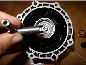
Hold shaft and in same time rotate (unscrew) impeller. In direction of the arrow.
