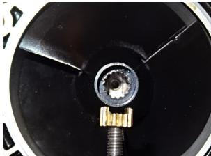
Security insert is in positin. Tighten it with philips (cross) screw.
