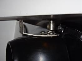
Unscrew 4 long screws, key 10 mm ( lower plate is removed for better visibility )
