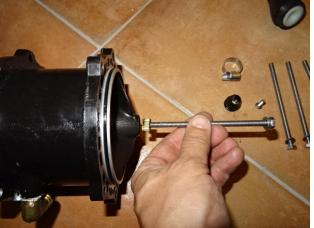
Remove brass security insert. Prepare tool to hold shaft. Pliers will also be good for this purpose.
