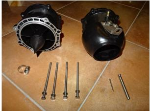
Unscrew plastic cone. If you are strong, by hand or with some big pliers. Don't squeeze plastic cone. Remove rubber seal.
