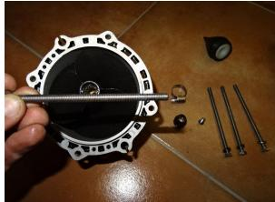
Screw long screw in the hole of brass security insert. Pull it out. Wiggle if needed.
