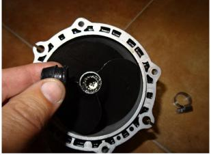
Unscrew – remove Philips (cross) screw.
