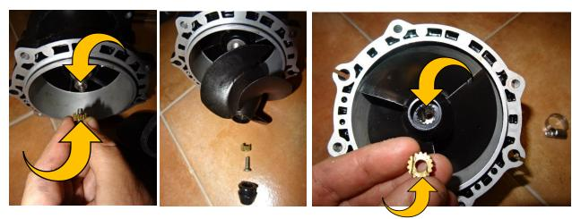
Security insert have function to prevent unscrewing of the impeller.
