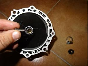
Note brass security insert below Philips screw. Take one of the long screws you removed previously.
